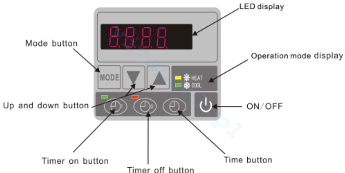
When the heat pump is running, the LED display shows the inlet water temperature.
