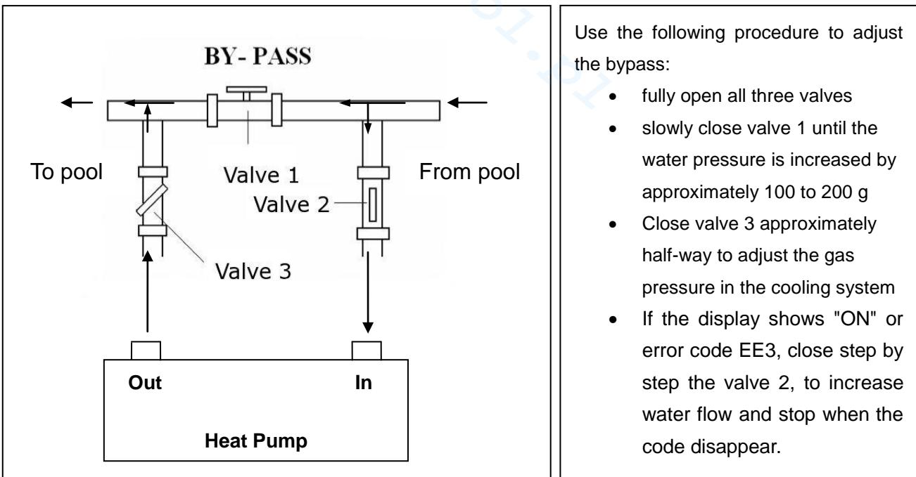
Optimal operation of the heat pump occurs when the cooling gas pressure is  $22 \pm 2$  bar.
